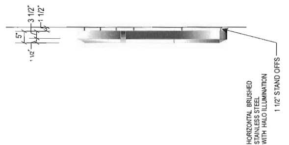
HORIZONTAL BRUSHED STAINLESS STEEL WITH HALO ILLUMINATION 1 1/2" STAND OFFS SIDE VIEW SCALE 1/2" = 1' 0"
