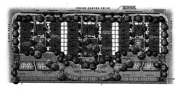
A 116-car parking lot (102 spaces are provided with carports) is located on the east half of the site and is separated from the courtyards by a meandering drive aisle that is accessed from Simms Road and San Rafael. Two trash/recycling enclosures are provided within the parking area. Open space is provided in three common area courtyards that are created between the rows of town-homes. These contain covered barbeque areas and one water play area for children in the center courtyard.
