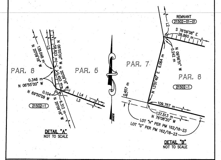
DISTANCES ARE IN METERS UNLESS OTHERWISE NOTED. MULTIPLY DISTANCES BY 1.00002594 TO OBTAIN GROUND LEVEL DISTANCES. TO CONVERT METERS TO U.S. SURVEY FOOT MULTIPLY **DISTANCES BY 3937/1200.**
