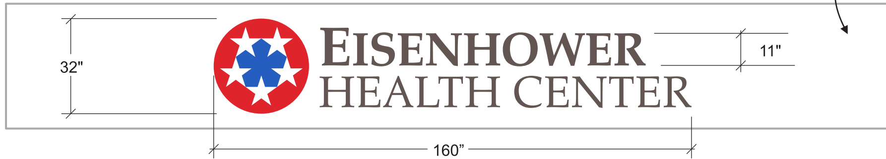
E EAST ELEVATION - SUNRISE WAY ALL ALUM LED REVERSE LIT CHANNEL LETTERS - LOGO FRONT / BACK LIT
