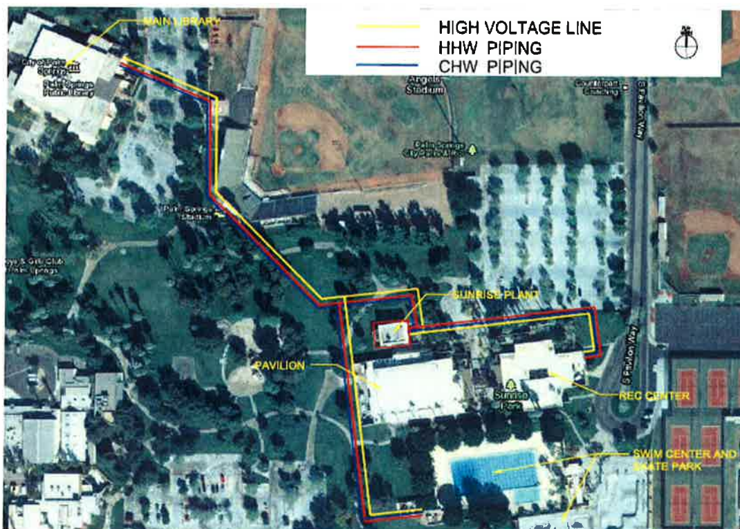
Figure 2-2: Sunrise Central Plant Infrastructure
