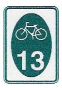
Figure 7: Numbered Bikeway Sign (MUTCD)
