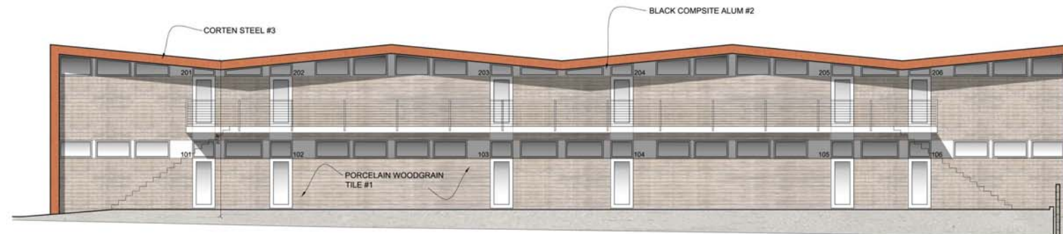
Building 1 - south elevation SCALE: 1/8" = 1'-0"
