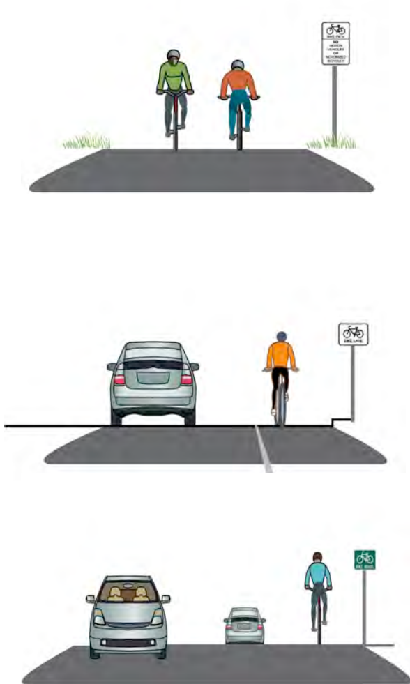
FIGURE 1 Class I (top), Class II (middle), and Class III (bottom) bikeways.
