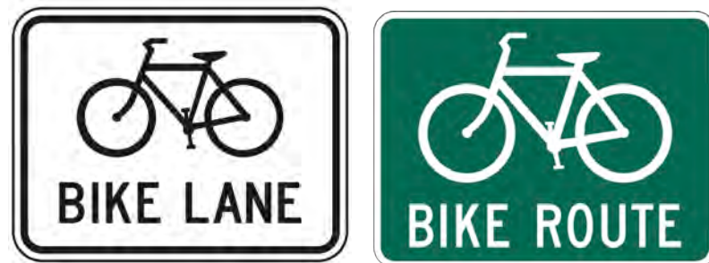
FIGURE 7 Bike Lane (R81) and Bike Route (D11-1) signs.
