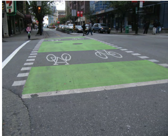
FIGURE 2 Cycle track intersection treatment.
