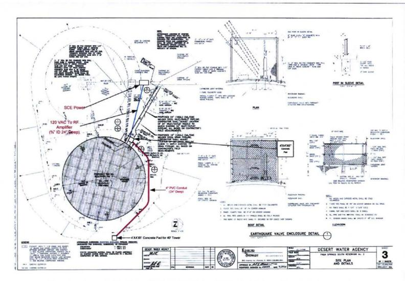
Concrete pad on west side of tank will have chain link fence and will adhere to the drawings Post & Sleeve Details. Tower will be a 40' self supporting Rohn 25G. No guy wires needed. Tower will have anti climb kit panels installed.
