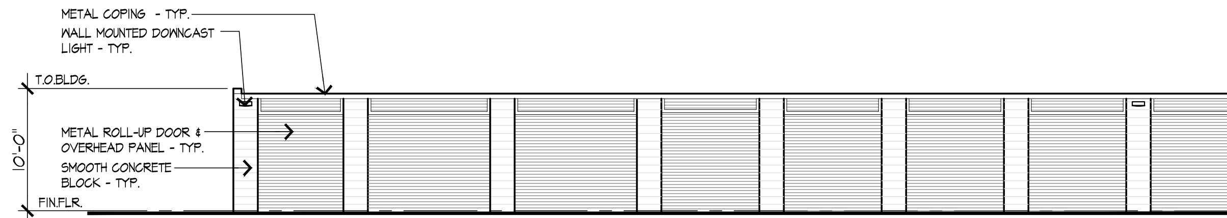
BLDG. C ENLARGED WEST ELEVATION (NORTH PORTION)
