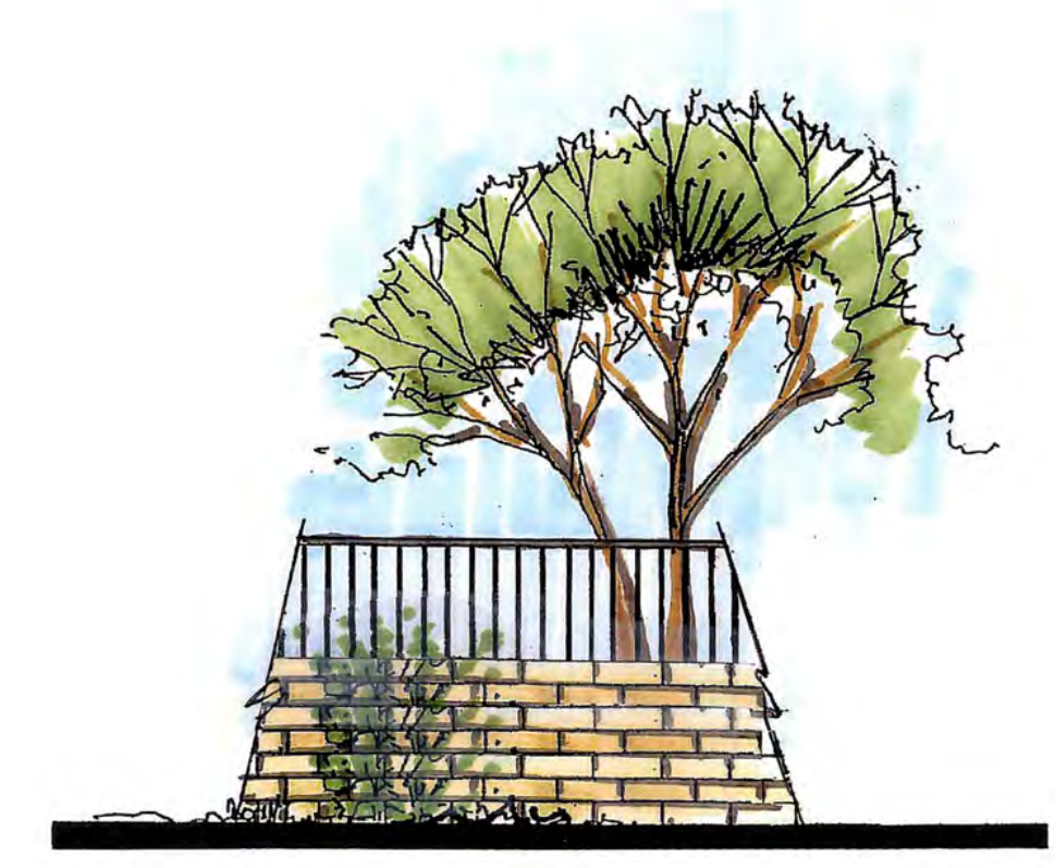
COMBINATION WALL & FENCE SLUMPSTONE BLOCK WALL AND TUBULAR STEEL FENCE. COMBINED 5' HEIGHT MINIMUM.
