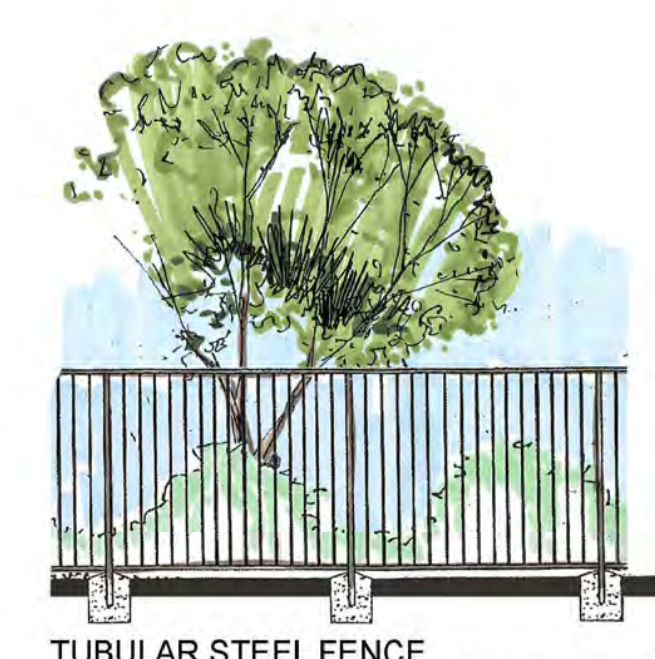
TUBULAR STEEL FENCE 5' HEIGHT MINIMUM
