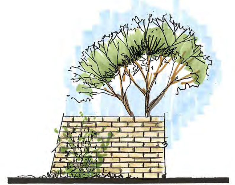
SLUMPSTONE BLOCK WALL SLUMPSTONE BLOCK WALL WITH SLUMPSTONE BLOCK CAP. 5' HEIGHT MINIMUM.
