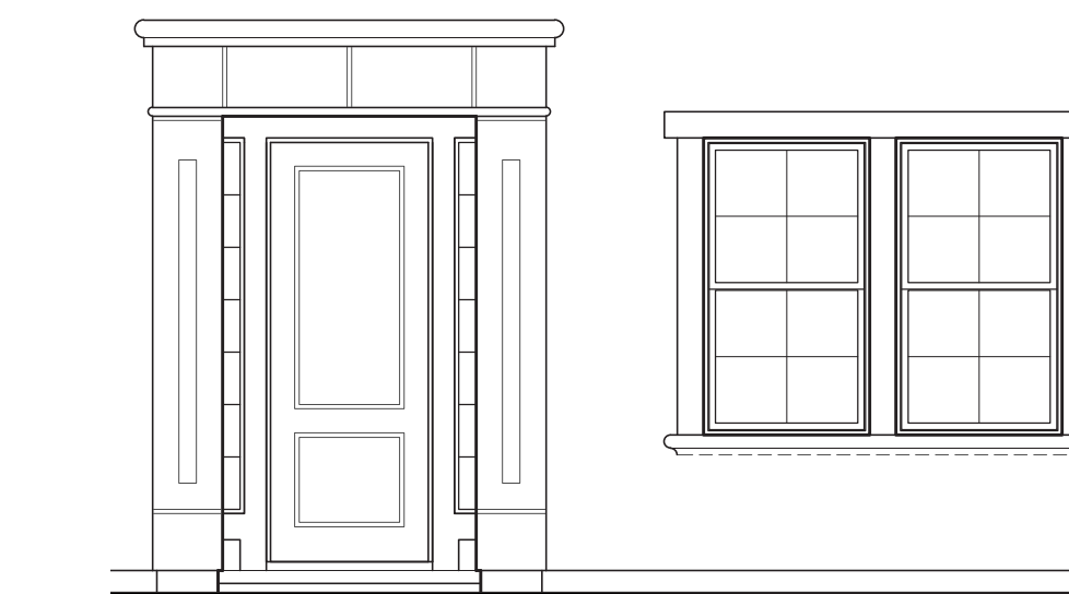
CEMENT-COATED FOAM SURROUND AT ENTRY
