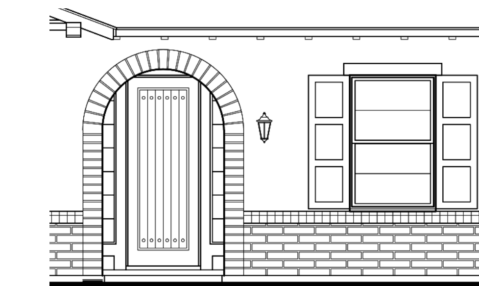
BRICK SURROUND ARCHED ENTRY AND COACH LIGHT. DECORATIVE SHUTTERS PER ARCHITECTURAL STYLE
