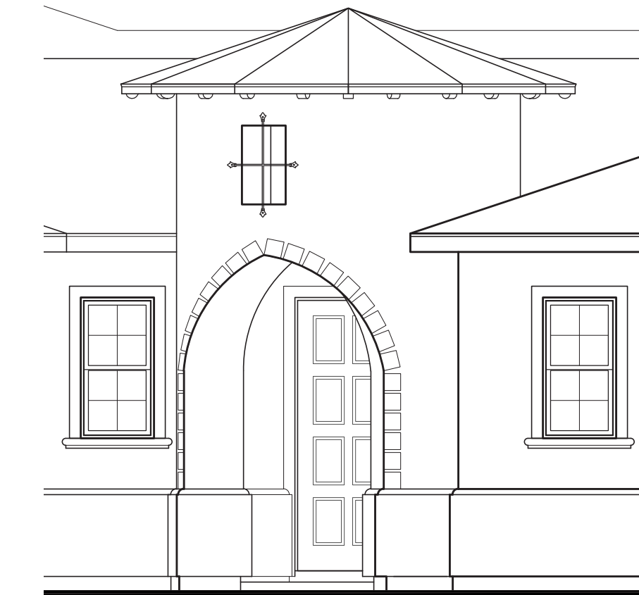
TURRET ENTRY INTO COURTYARD, DECORATIVE TILE ACCENT SURROUND ARCHED ENTRY, WOOD RAFTER TAILS AND 25% BOOSTED "S" TILE ROOF
