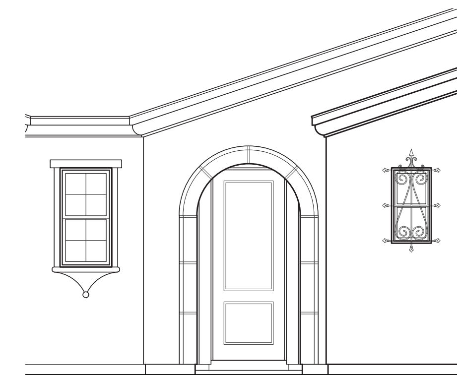
CEMENT-COATED FOAM SURROUND AT ENTRY. DECORATIVE METAL GRILL ACCENT AT WINDOW
