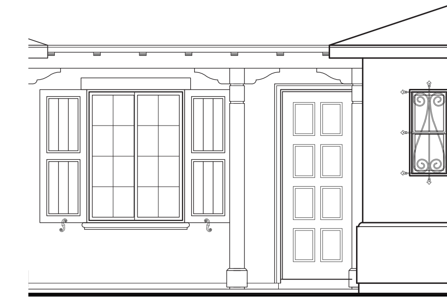
POST WITH SHAPED BRACE AT PORCH, WOOD RAFTER TAILS AND 25% BOOSTED "S" TILE ROOF
