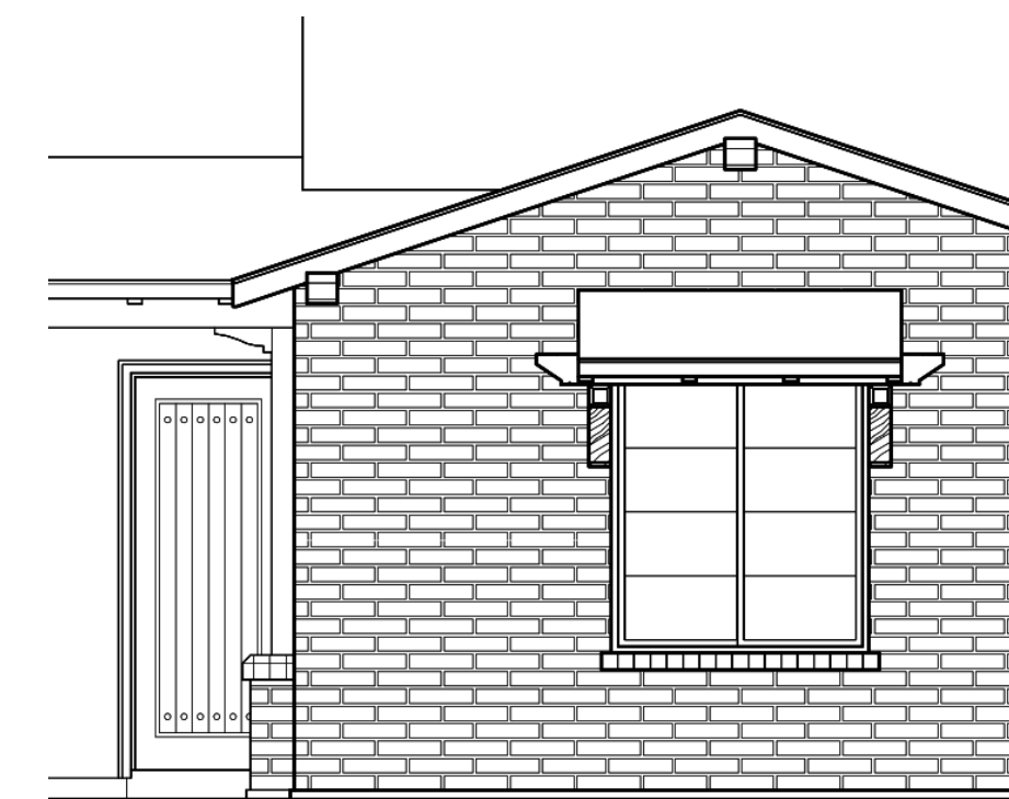
BRICK VENEER WALL ACCENT AT PORCH ENTRY. RAFTER/TAILS AT SELECT AREA WITH WOOD POSTS, SHAPED BRACE AND BRICK VENEER BASE
