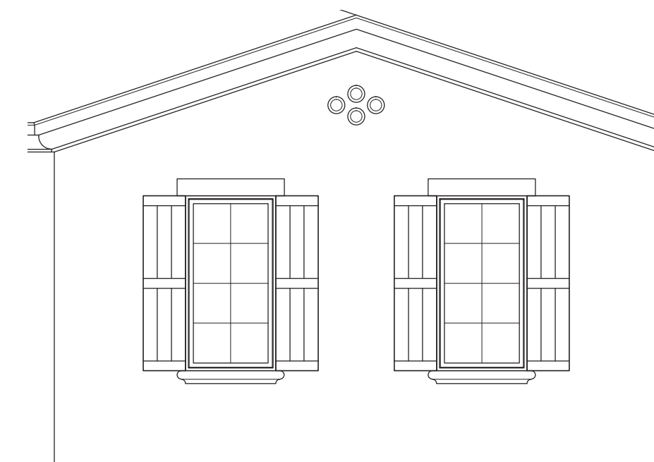
GABLE WITH FOAM ACCENT PIPES. DECORATIVE SHUTTERS WITH SCULPTED STUCCO OVER RIGID FOAM SILL TRIM
