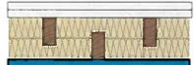
QuietRock on one side 2 layers 5/8" Type X on the other
