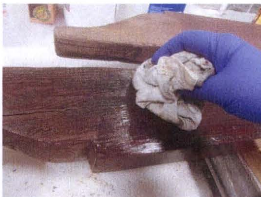
18. Dabbing with rag to add texture. (Not applicable for painted finish)
