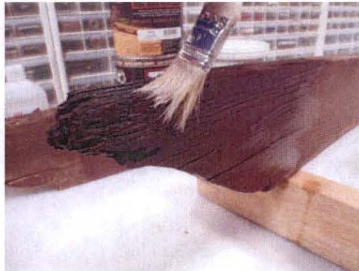
4. Application of borate-based wood preservative.
