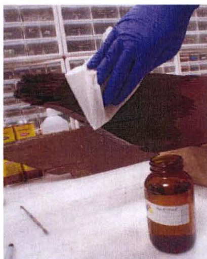
6. Removal of excess at surface with acetone.
