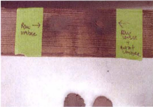
7. Color tests using dry pigments to integrally pigment WoodEpoxy epoxy fill (Not applicable if painting.)
