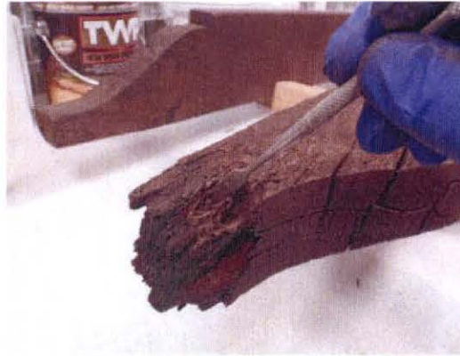
8. Filling voids with WoodEpoxy epoxy filler.
