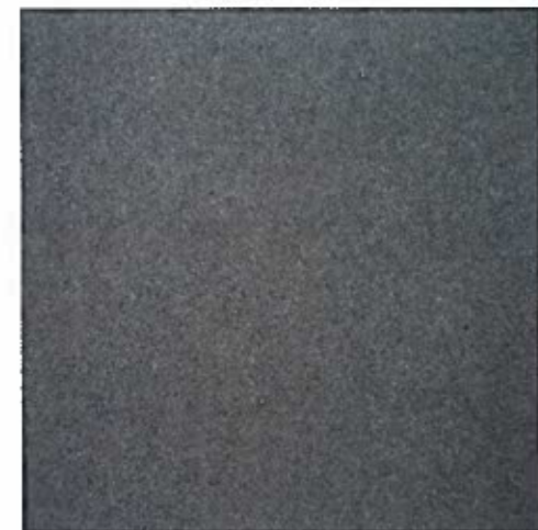
7 H-1 CONCRETE HARDSCAPE, NATURAL GRAY W/ACID ETCH FINISH
