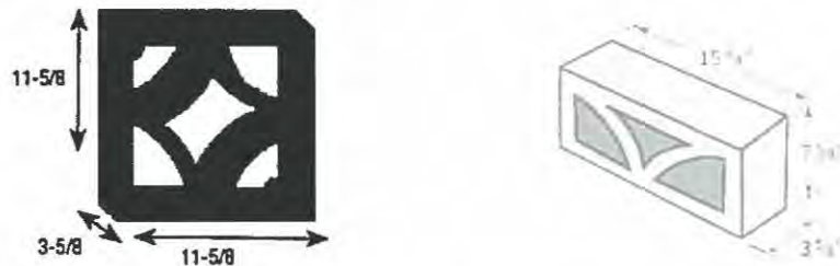
Empress (on left) and Four Square (on right) pattern concrete screen blocks
