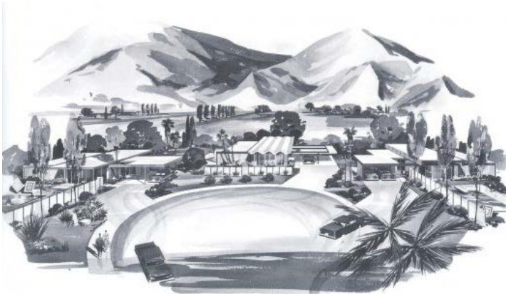
This drawing shows the three rooflines: flat, clerestory, and folded plate giving the neighborhood an interesting visual appearance. Source: "AD Classics: Steel Pre-Fab Houses / Donald Wexler," ArchDaily , August 20, 2011.
