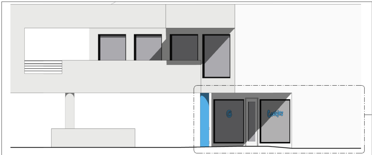
Image 1.4 Proposed Paint Application – East Elevation
