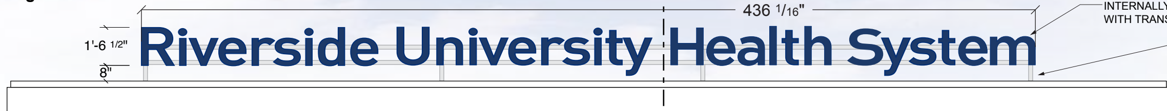
1 2 INTERNALLY ILLUMINATED CANOPY SIGN DIMENSIONAL LETTERS SCALE: 1/4" = 1'-0"
