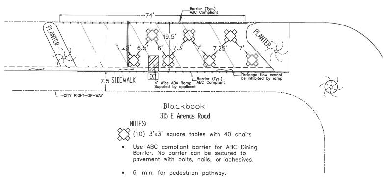
4'-Wide Ramp down into parklet will comply with ADA requirements. Drainage flow cannot be inhibited by the ramp.
