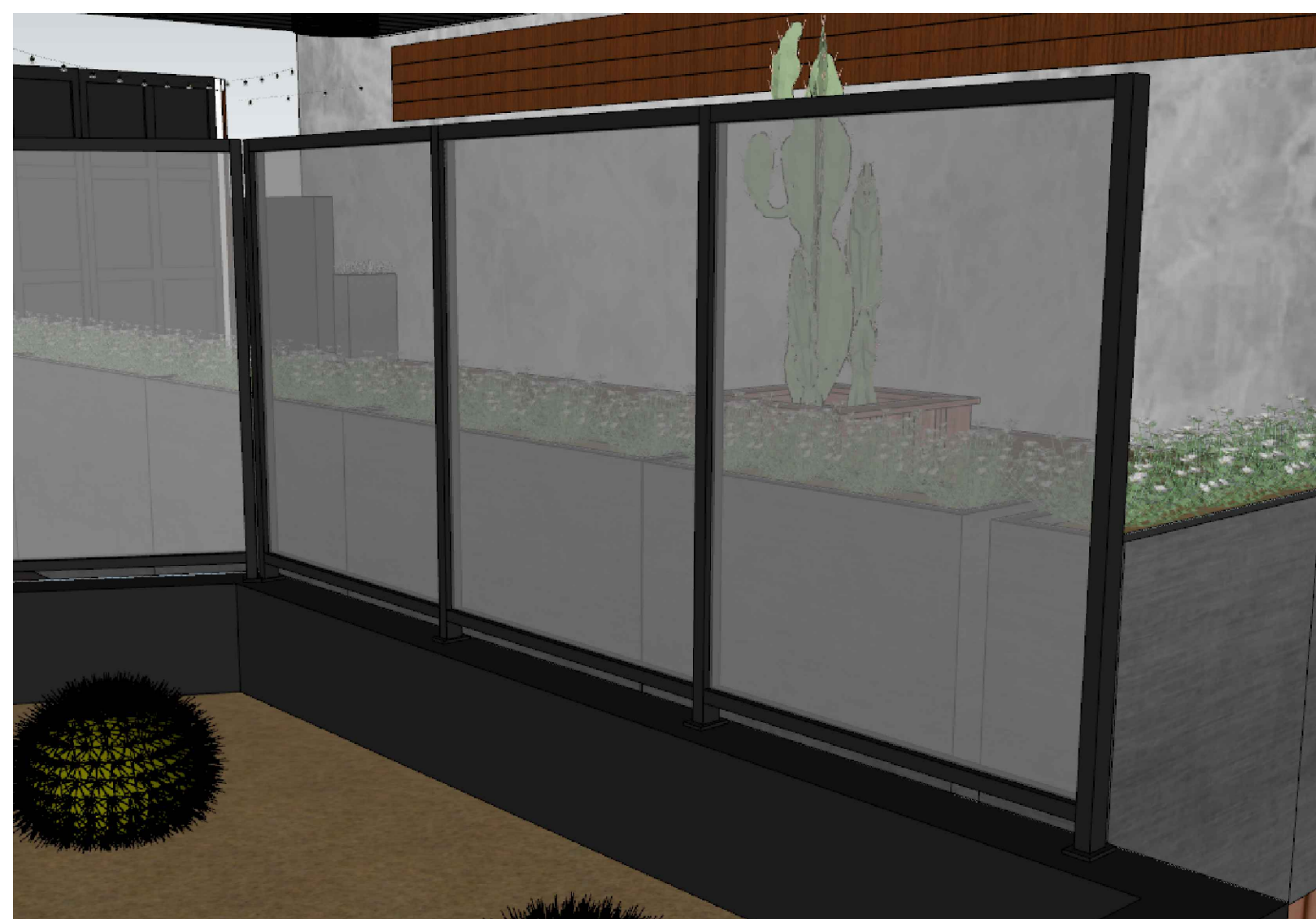
48" HIGH GLASS WIND PARTITIONS ON METAL FRAME
