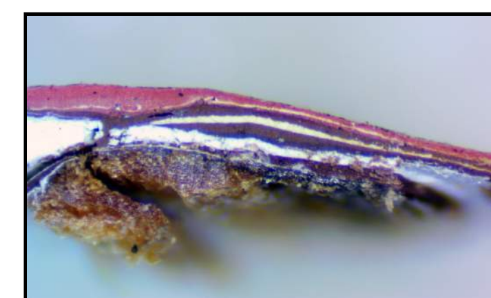
SAMPLE NO. 17 WOOD DOOR FRAME 215A 11. (E) MODERATE VERMILLION 10. MODERATE VERMILLION 9. WHITE 8. MODERATE VERMILLION 7. DARK BROWN 6. WHITE 5. DARK BROWN 4. BLACK 3. WHITE 2. DARK BROWN 1. WHITE (PRIMER)
