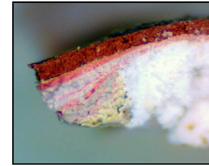
SAMPLE NO. 45 WALL FINISH AT SOUTH ATMOSPHERIC WALL, AT ROW 26 10. MODERATE VERMILLION 9. DARK YELLOW OCHRE 8. DARK PINK 7. LIGHT PINK 6. MEDIUM PINK 5. LIGHT PINK 4. DARK PINK 3. LIGHT PINK 2. MEDIUM PINK 1. YELLOWISH-WHITE/CREAM
