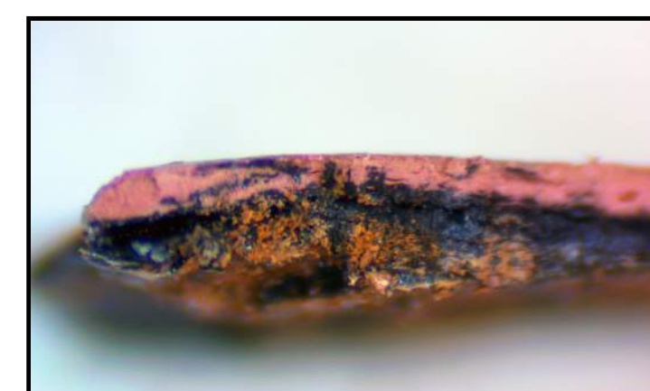
SAMPLE NO. 14 METAL GRILLE AT WIN. 103A 6. (E) MODERATE VERMILLION 5. MODERATE VERMILLION 4. BLACK 3. BLACK 2. BROWNISH-BLACK 1. REDDISH-ORANGE (PRIMER)
