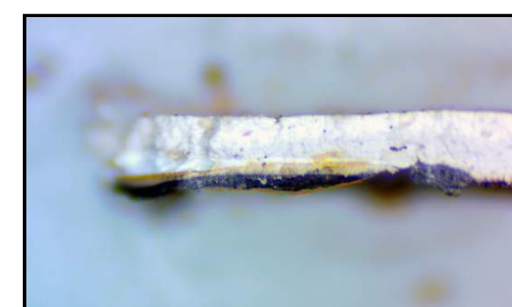
SAMPLE NO. 15 STEEL SASH AT WIN. 103A 8. (E) OFF-WHITE/CREAM 7. OFF-WHITE/CREAM 6. WHITE 5. YELLOW 4. WHITE 3. YELLOWISH-WHITE/CREAM 2. BROWNISH-BLACK 1. REDDISH-ORANGE (PRIMER)
