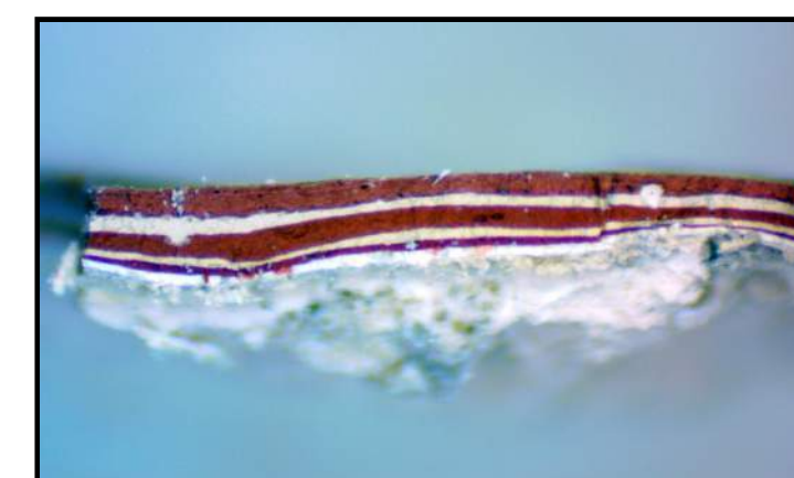
SAMPLE NO. 02 EXTERIOR CONCRETE WALL, WEST ELEV. ARCH BORDER TRIM 7. DEEP VERMILLION/RED 6. WHITE 5. DEEP VERMILLION/RED 4. WHITE 3. DEEP VERMILLION/RED 2. WHITE 1. YELLOWISH-WHITE/CREAM
