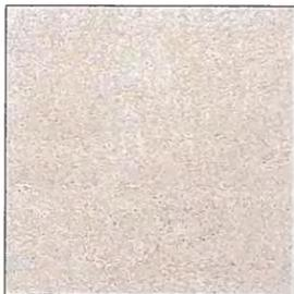
**EF-1** WHITE STUCCO; 3 COAT PORTLAND PLASTER CEMENT SYSTEM w/MESH & ACRYLIC COATING BETWEEN BROWN & FINISH COATS; SMOOTH SAND FINISH; "DOVE GREY" BY LA HABRA OR SIMILAR
